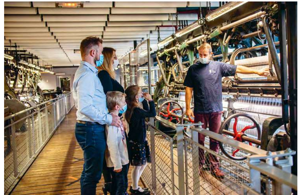
Professional demonstration of Calais-Caudry® mechanical lace weaving on Leavers looms.
