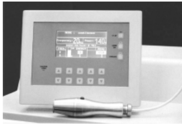
Figure 3 : "Smart Clean" Laser with details of the display, optical cable and of the handpiece.
