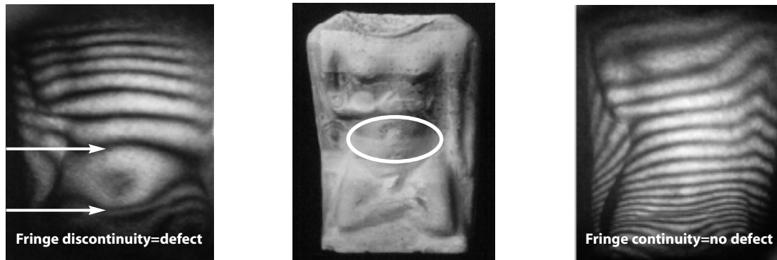
Figure 2 : A ceramic statuette in the middle examined with holographic interferometry at left prior and at right after the laser cleaning. The circular pattern reveals a characteristic detached region due to lost of adhesion of the upper pigment layer to the solid whereas the continuity of fringes observed after the cleaning confirms successful restoration process.
